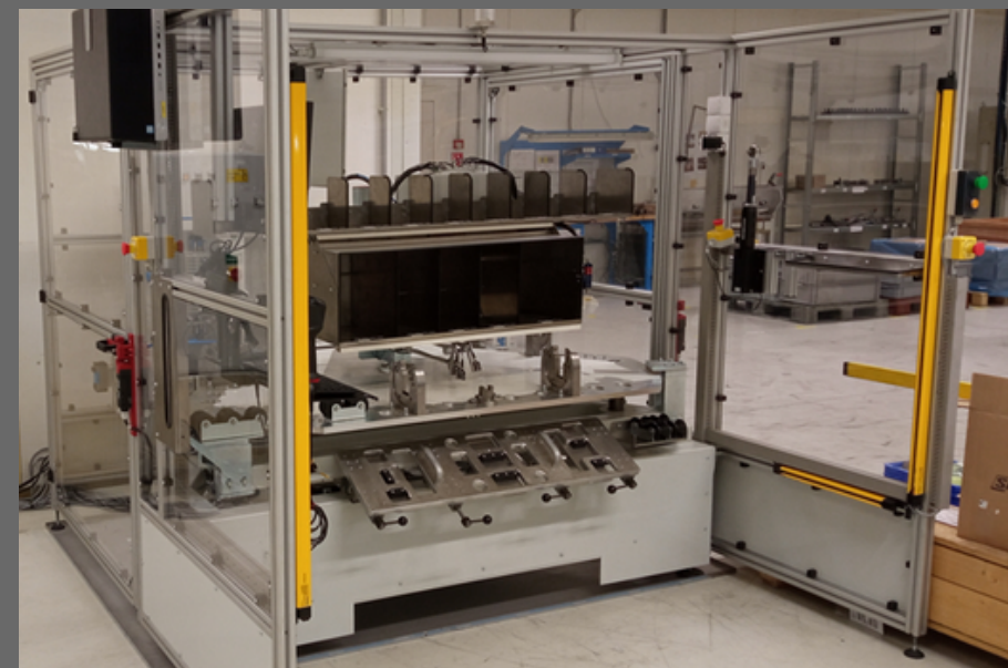
Common Rail assembly and testing rotary table
